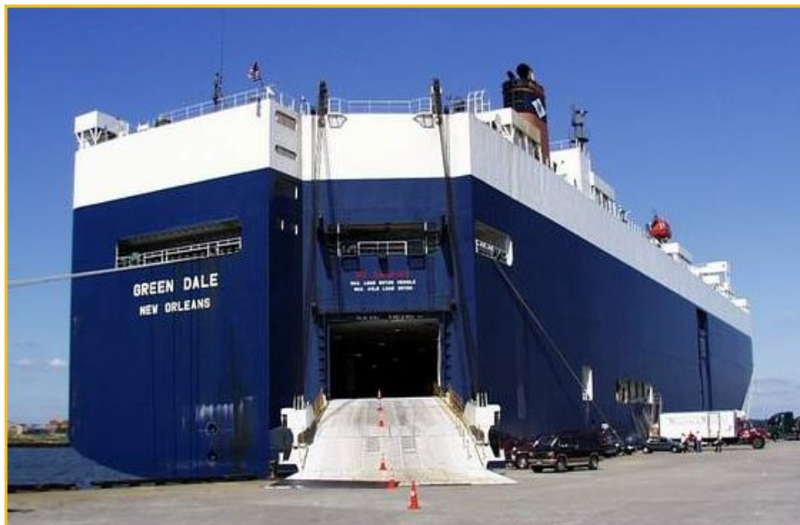
Waterman Steamship Corporation's US-Flag Pure Car / Truck Carrier (PCTC) Roll-on/Roll-off (Ro/Ro) Vessel.
